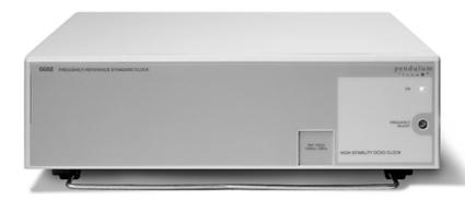
The Pendulum Frequency References; model 6689 with a Rubidium clock and model 6688 with a high-stability oven-controlled crystal oscillator, are designed for use in test systems, where a very high stability frequency reference is required and where multiple instruments or testers need to be supplied.
